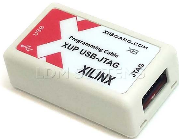
Figure 1. General view of the download cable XB-XUP USB-JTAG
